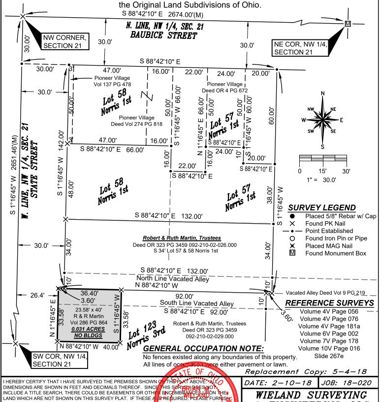
HOVVIN ON THE FRAT CABOVE THE NECESSARY INFORMATION. THE BEARINGS AND DISTANCES ARE BASED ON STATE PLANE COORDINATES, SPC83, ZONE-OHIO RECORDED IN VOL. 10V PAGE 031 OF THE WILLIAMS COUNTY SU
